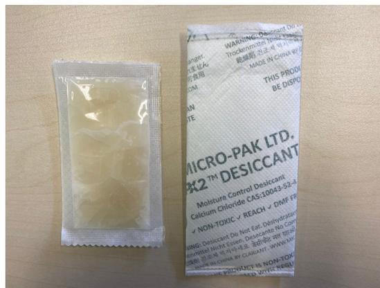
Fig. 2 Calcium chloride packaging consists of an inner plastic pouch and an outer non-woven layer
